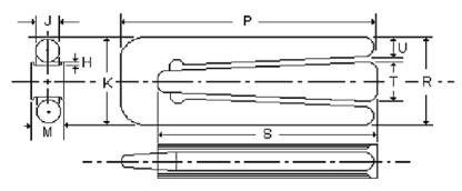
\*Drawing depicts typical dimensions (Dimensions are all in mm) E – As Supplied / S - After Free Recovery / S – Adhesive Internal Length / P – Length as per Requirement / T - Thickness
