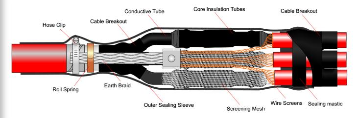
\*A 12kV Joint has a dual wall insulating/conductive tube above the stress control tube.
