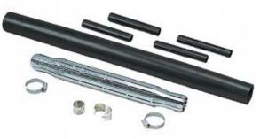
Utilising REPL Heat Shrink tubes, these joint kits are suitable for jointing armoured cables with XLPE or PVC insulation up to 3300v. Due to their compact dimensions and small profile they are ideal for use in confined areas such as cable trays, but can also be used in direct buried applications and are suitable for vertical cable runs.
