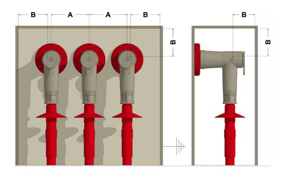
Ensure that the minimum clearances are according to the table below for the required voltage level, these dimensions are in accordance with IEC 60071-1 to 71-3
